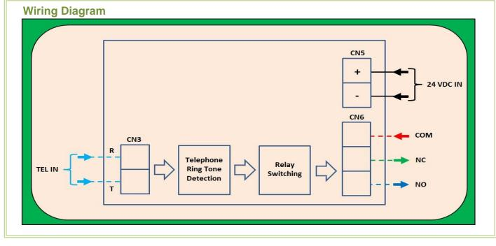
Telephone ring detector module with dry contact output, DC 24V input with snap-in DIN rail mount bracket. The module allows the telephone to activate a peripheral device such as a light beacon when the ring voltage (or tone) is present.
