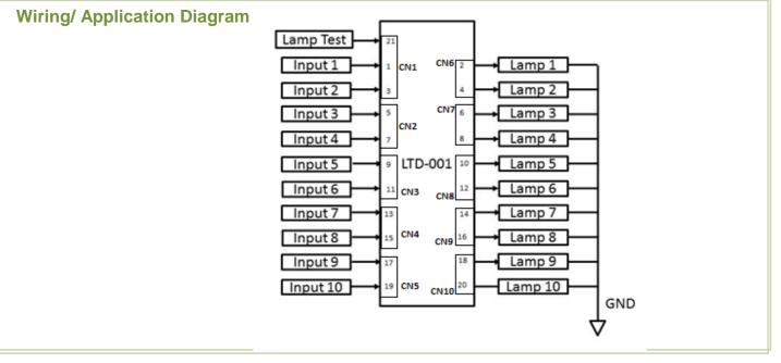
Diode Board is generally for use in connection with lamp test panel. It comes with 10 inputs and 10 outputs. No additional screw is required to install the diode board, no additional wire is needed for the assembly, and the compact size with built-in input and output terminal blocks for easy wiring and termination.
